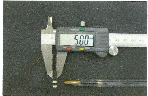
Two samples that are 5mm in depth are needed from each piece. 每件器物需鑽取兩個 5毫米深的核心樣
