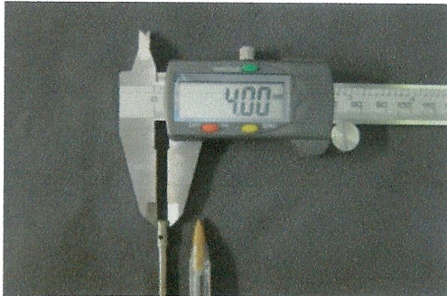
The drill bit used for core sampling is 4mm in diameter. 以直徑4毫米的鑽嘴進行核心取樣。
